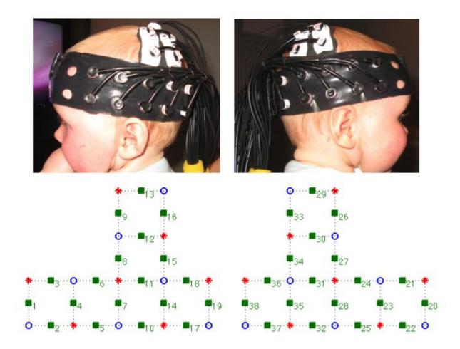
**Fig 2**. fNIRS headgear and channel layout. Top images show photo of left and right source/detector arrays as placed on infant head. Bottom images show location of sources (red stars), detectors (blue circles) and resulting channels (green squares).
